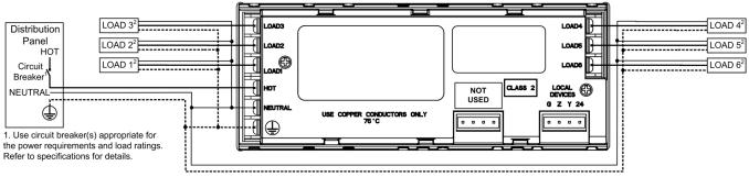
2. CLS-EXP expansion modules can be used in place of any or all loads shown above. Refer to expansion module documentation for wiring details.
